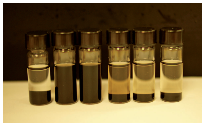
Figure 7. Images of GO and GO-PTh nanocomposite dispersions in DMF. From left to right: GO, and GO-PTh samples prepared at 70 °C over 24 h, 12 h, 4 h, and prepared at 50 °C and room temperature over 24 h, respectively.
